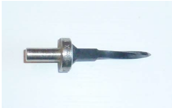
Figure 37 Stanley Screw Mate from the 1960s. It countersinks the head flush to the wood, however it could be designed to countersink deep enough for a bung.
