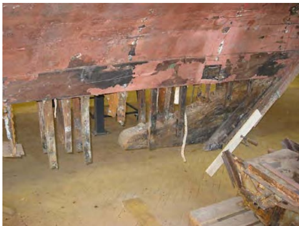
26) Original oak crook sternpost knee. Note that the Wooden Boat Center's construction floor is end-grain, wood blocks. (Pedrick)
