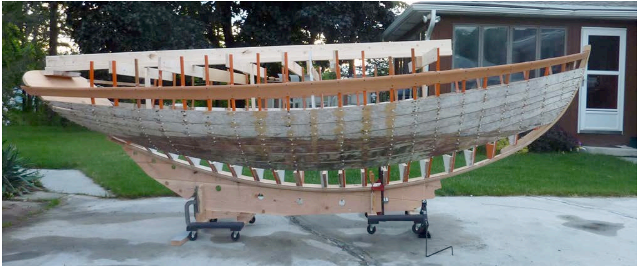
Figure 25 Profile view showing the flat of the sheer in the midsection. The old planking is attached to the boat with wire ties around the frames because I didn't want to screw into the new frames until I was actually screwing in the new planking.
