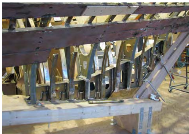
27) New sternpost knee in bronze. It includes female-threaded sockets for bolts through keel and sternpost. (Pedrick)
