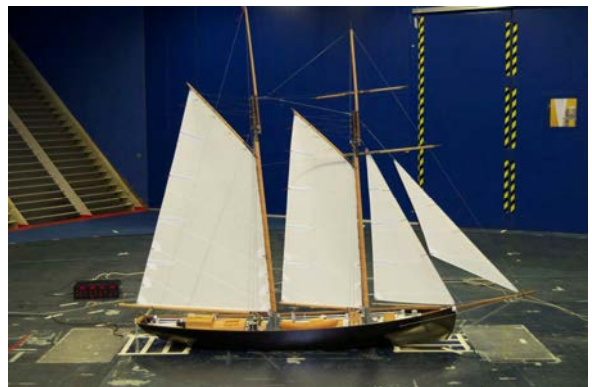
Figure 23 – S1-JT-k-h4 sailplan layout (smaller jib at lowest height)
