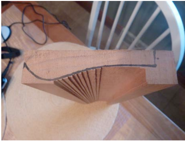
Figure 23 The router creates a stair-step pattern close to the desired profile. Reminds me of Simpson's rule for calculating the area under a curve.
