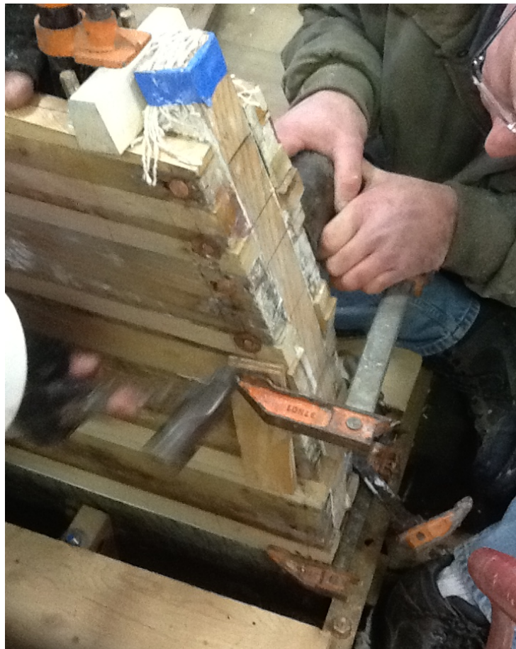
Figure 10 Riveting of original trunk sides re-using original roves
