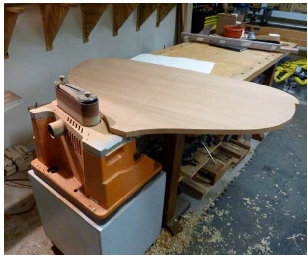
Figure 16 Cleaning up the overall shape of the transom prior to making the edge bevel.
