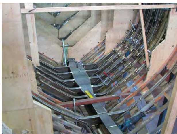
35) Mast step, web frames and aft end of bow girder. Full station molds amidships are shown here, October 2010. (Pedrick)
