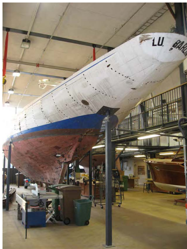
12) In the construction hall, March 2009, before truing up the sheerline (Pedrick)
