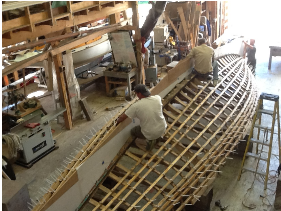
Figure 3 Keel rocker patterns in place and structure bent to fit
