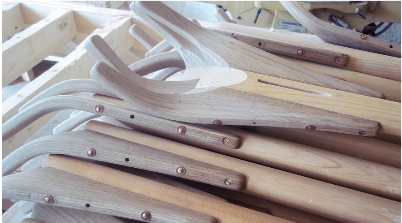
Figure 1 – Gaffs with jaws assembled following CNC machining to shape the jaws and cut the slots for the throat halyard tangs; just one of the production line operations enabling completion all of the woodworking in just six weeks.
