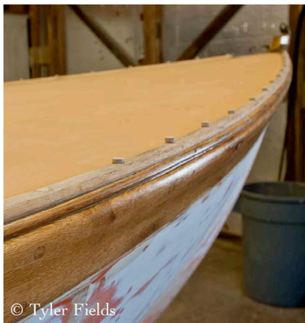
Figure 4- Foredeck planking was refastened and canvassed. Replacement of original toerail covering edge of the finished canvas. Note original patina preserved in brightwork.
