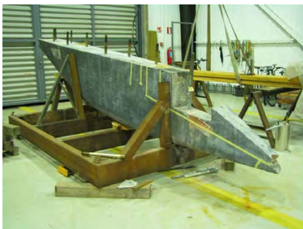
44) A pocket had been removed from the original keel casting, apparently to correct flotation in 1937. Tape marks the boundary of additional lead removal required now by the added engine and systems. (Pedrick)
