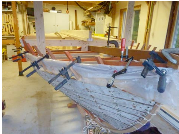
Figure 34 A similar steam set up was used for the sheer strakes. This photo demonstrates how parts can be clamped in place with the bag still in place slowing down the cooling.
