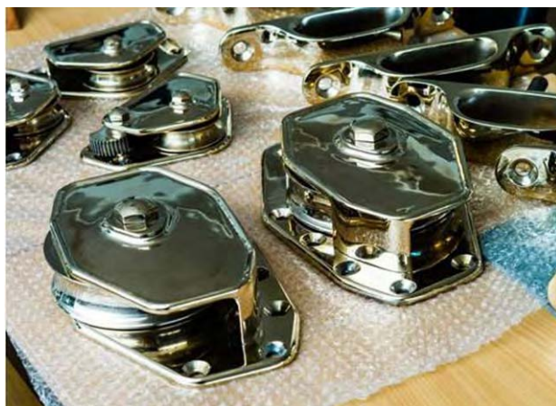
57) Footblocks designed by Pedrick Yacht Designs and manufactured by Blockmakers Ording. (Skogström)
