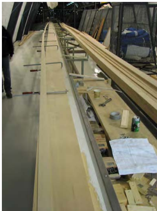
77) Spar bench on left, in loft at Wooden Boat Center. Tapered staves are at right. November 2011. (Pedrick)
