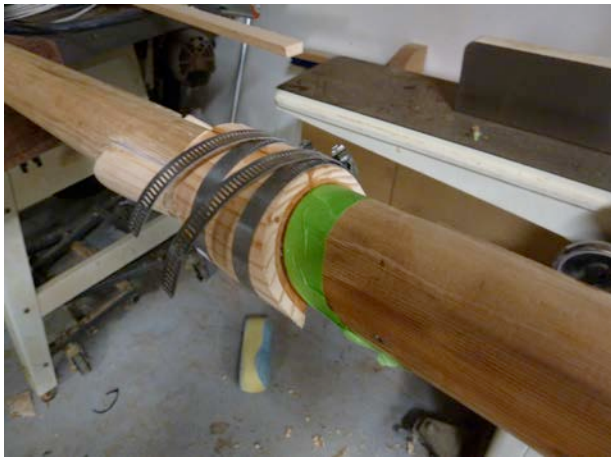
Figure 21 Hose clamps are useful in securing the hounds while the epoxy dries.
