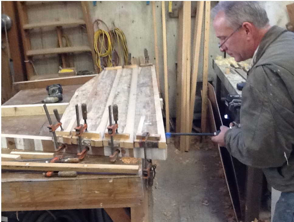
Figure 9 John Taylor drilling repaired centerboard trunk sides for through bolts
