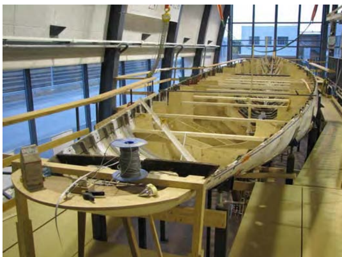
34) Stations molds cut back in the bow, where bronze frames have been fitted. Full molds are in place from amidships aft, October 2010. (Pedrick)
