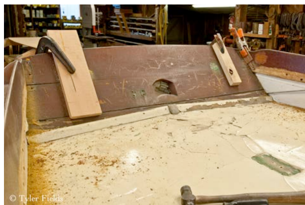
Figure 3- Sample of issues for attention: cracked transom, flaking varnish, peeling deck “canvas”.
