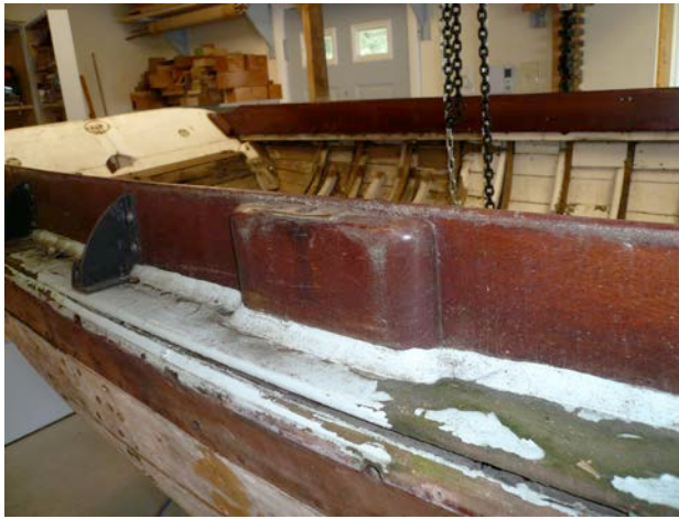
Figure 6 Photo showing the amount of caulk used to prevent leaking around the coamings. Also note the block used for the oarlock socket, typical of later boats. Metal support pieces were added by a previous owner to support the coamings as well.
