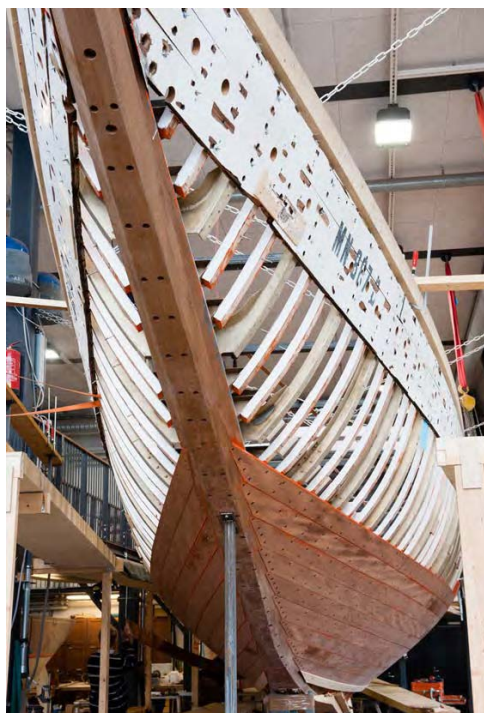
38) All framing completed. New lower planks. Original upper topsides still in place, early 2011. (Skogström)
