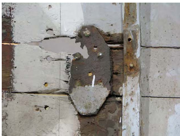
22) Rusty butt plate and rotted hull planks in topsides aft. (Pedrick)
