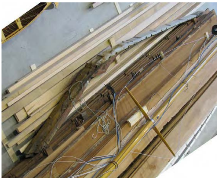
24) Original stern timbers, made in three parts. The stern post on the left rises from the wood keel. The counter timber is relatively straight on the right. They are ship-lapped onto the curved horn timber in the middle. It is resting on spruce for the mast. (Pedrick)
