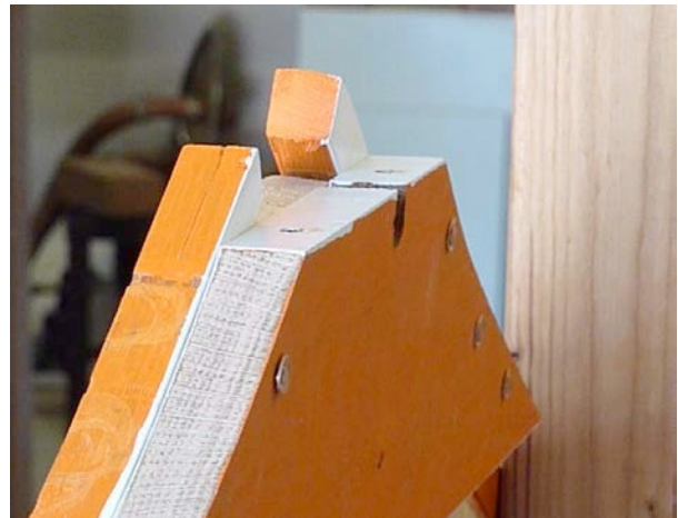
Figure 36 Painting before assembly. The mating surfaces are primed and painted before riveting the parts together. After sawing the frames flush, the end grain on the frames and the floors receive the same treatment.
