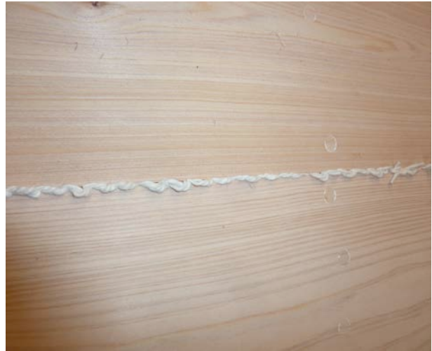
Figure 31 Looping in a second time. After stitching the first loops in half, we “make” the seam by pushing the caulking even with the seam, like in the center of this photo. The caulking is then “set” in with roller similar to a pizza cutter or pushed in with a putty knife or fine blade caulking iron.
