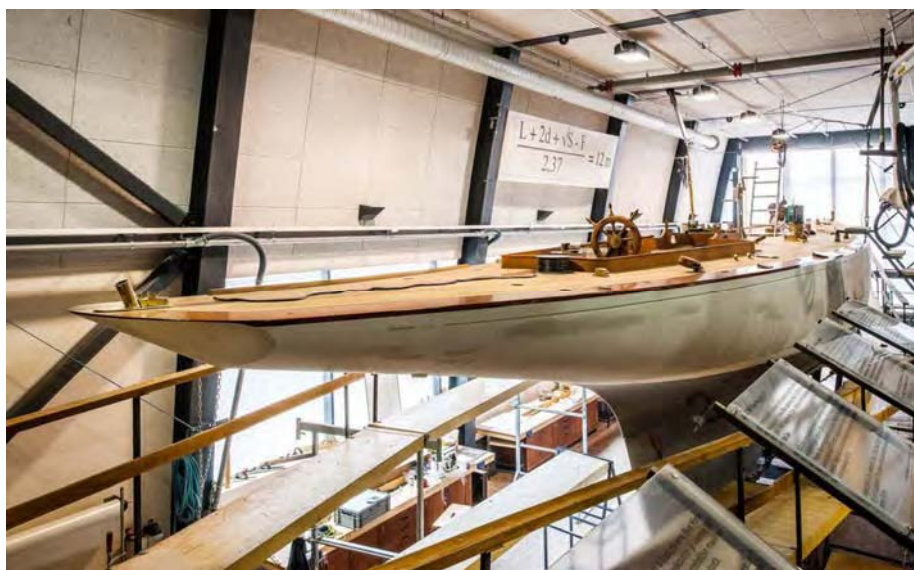
9) In the final stages at the WBC, April 2014. Deck fit-out, varnishing and installation of interior components are nearly complete. Work in progress is visible from the sidewalk outdoors and a viewing bridge to the right. Storyboards on the viewing bridge describe the project. (Pedrick)
