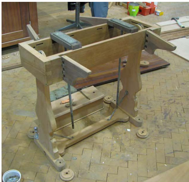
67) BLUE MARLIN's original drop-leaf table being restored. Pendulum weights are placed upside down. They go in the box on the floor behind the table. (Pedrick)
