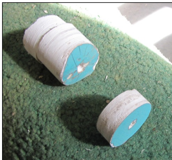
7.) ARION hull cores; upper core is hull centerline, lower core is from about the turn of the bilge.
