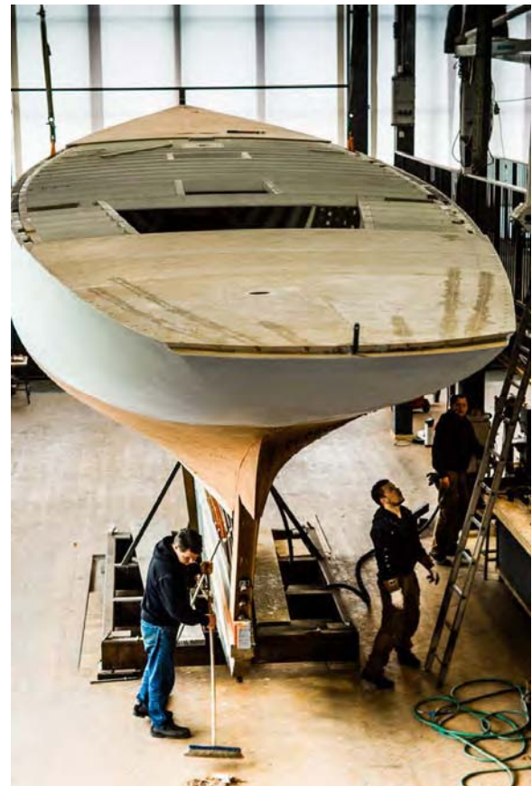
63) Hull soon after setting it onto the ballast keel, early 2012. Plywood deck is installed at the bow and stern. (Skogström)
