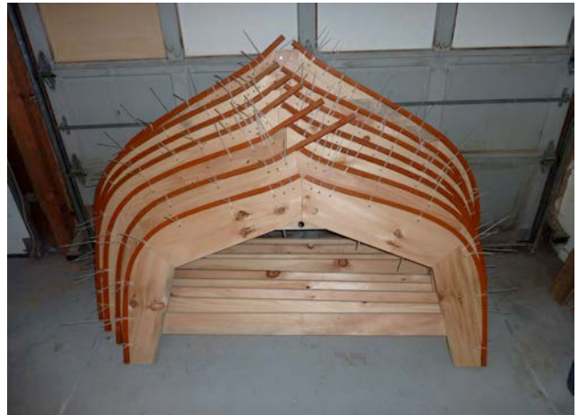
Figure 7 Frames on the molds after steam bending; notice the use of wire ties.
