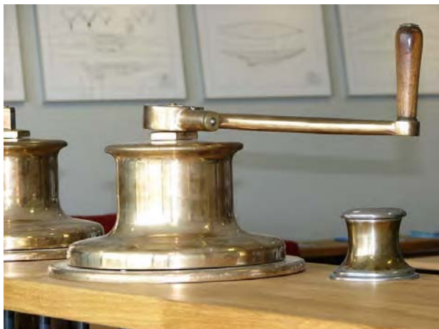
54) Antique British winch used as prototype for BLUE MARLIN's new, custom top-action winches. (Pedrick)
