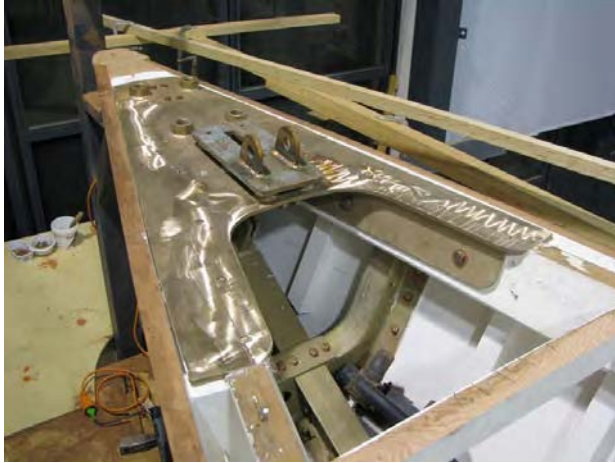
61) Breastplate with flanges bolted through the shear clamps. Watertight sockets receive bolts to secure the removable anchor roller, as well as the jib tack plate. (Pedrick)
