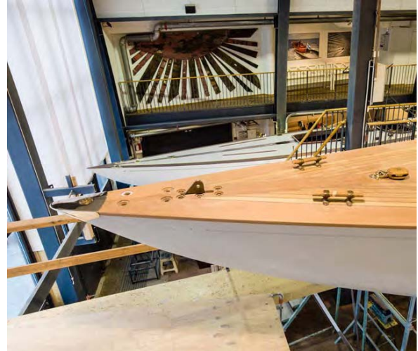
62) Holes through the forward end of the deck will receive threaded sockets that secure into the breastplate sockets. There is an additional anchor roller socket in the stem cap. The headstay tang is connected directly to the centerline girder. Note the Six Metre and rudder sculpture in the background. (Skogström)
