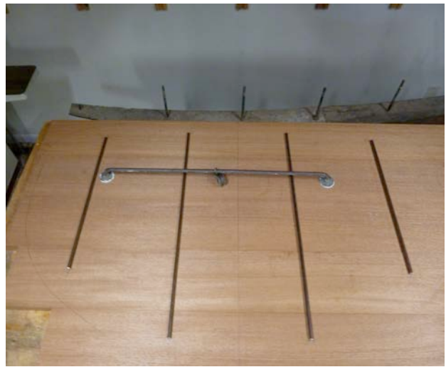
Figure 15 Aligning the bronze drifts so they don't interfere with the traveler. This view is from the aft end of the transom. Notice the traveler is offset to the port side of the boat because the mainsheet block is to the starboard side of the tiller. This compensates so that no adjustment of the sheet is necessary when changing tacks.
