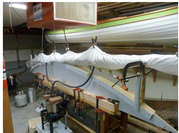
Figure 33 Steam set up for the keel plank.
