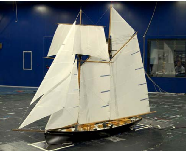
Figure 5 – 1:15 scale model at 60° AWA
