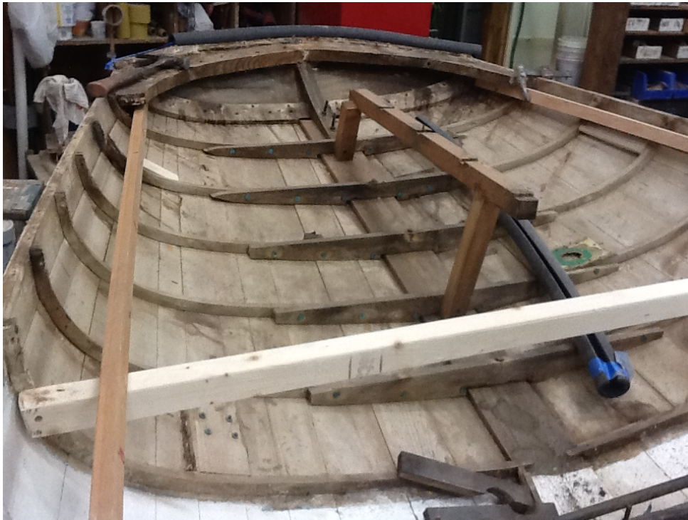
Figure 8 Showing original "whitewash" used as a sealer/primer. Photo is of the area inside a watertight bulkhead in a 1914 BB15 (HMCo #731) that is being restored alongside MINK. The finish is typically found in all areas of the hull not finish painted. MINK will get the same treatment.
