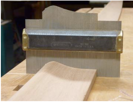
Figure 3 Profile gauge used to verify the shape of the sheer strake.
