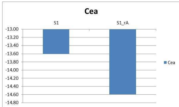
Figure 61 – Rake effect on center of effort longitudinal position (4 Lowers)
