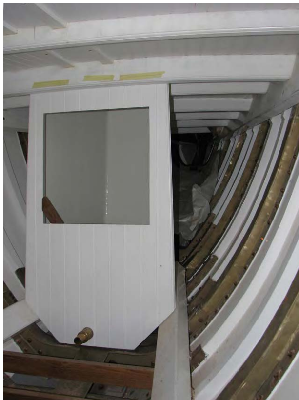
60) Deck beams in bow completed, early 2012. All beams are beaded on their lower edges. Anchor rode locker has large opening for acrylic hatch. (Pedrick)
