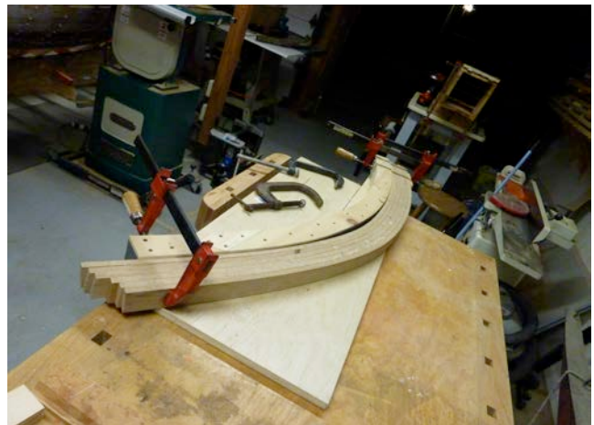
Figure 8 Unglued stem laminations clamped to the form after steaming in an effort to pre-curve them to facilitate glue up.
