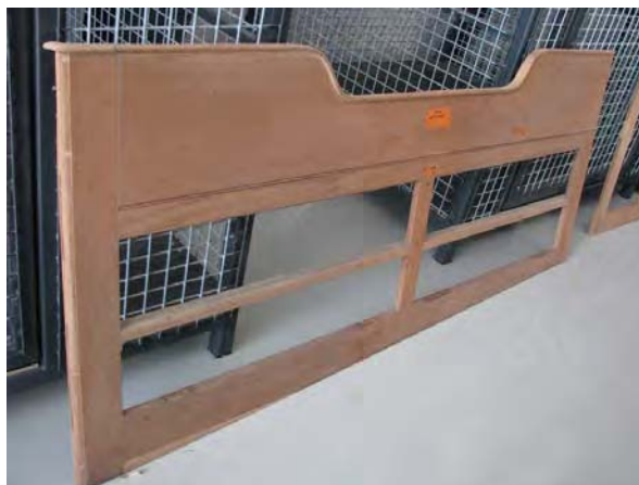
65) Berth front from original owner's cabin. It is being re-used as a pilot berth front. The original settee fronts in the salon are being re-used. A matched set of new panels has been made for the midships settees and pilot berths. (Pedrick)
