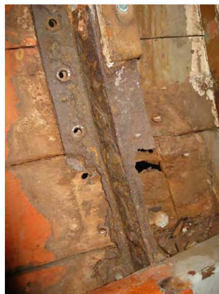
21) Steel Z-frame in topsides forward, with both flanges rusted away. (Pedrick)
