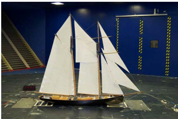
Figure 20 –S3-JT-h1 sailplan layout (Jib topsail higher)
