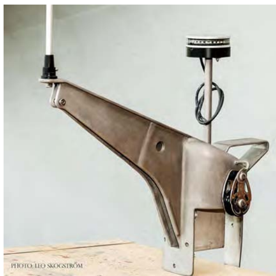
78) Masthead fitting with sheave and pin for a two-part main halyard; also, backstay crane, VHF antenna, LED masthead light and base for wind instruments. Gantline block is a stock, practical concession, difficult to be seen from the deck or dock. (Skogström)
