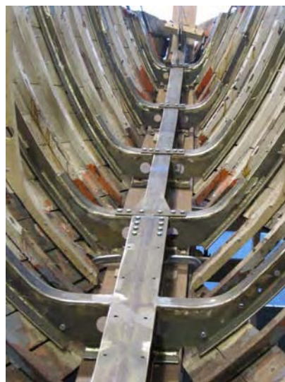
36) Bow girder, floors and bronze frames. Original bent frames are still in place, October 2010. (Pedrick)
