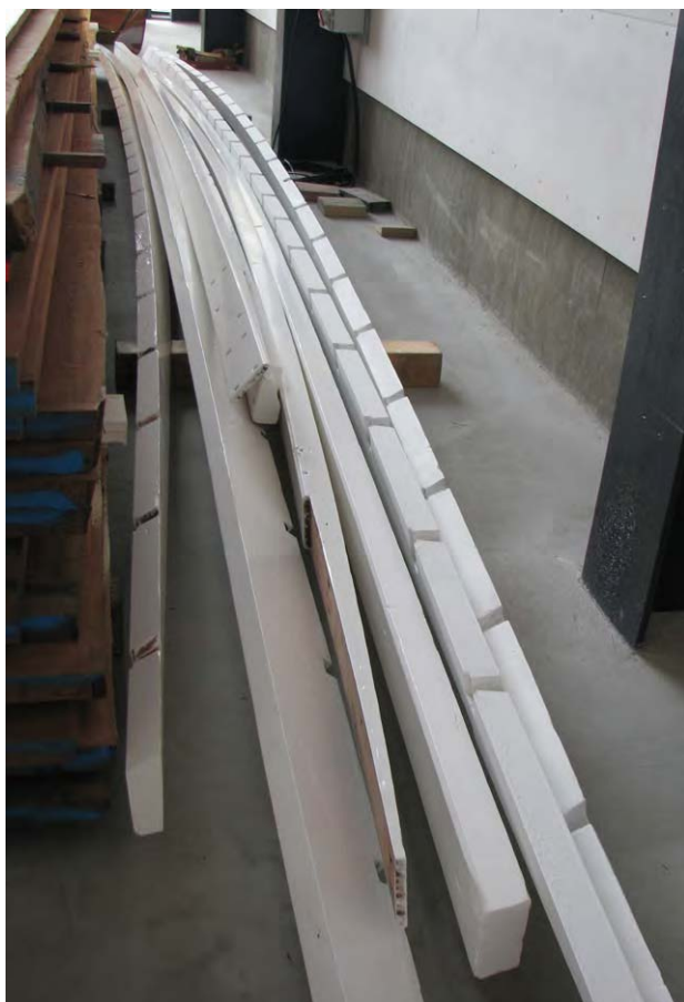
25) Original sheer clamps and bilge stringers, restored and waiting for reassembly. Mid-2010. (Pedrick)
