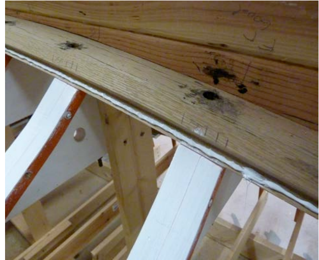
Figure 28 Sikaflex 291 on the garboard rabbet. Also notice the frames and floor timber end grain have been primed and painted where they will mate with the planks.
