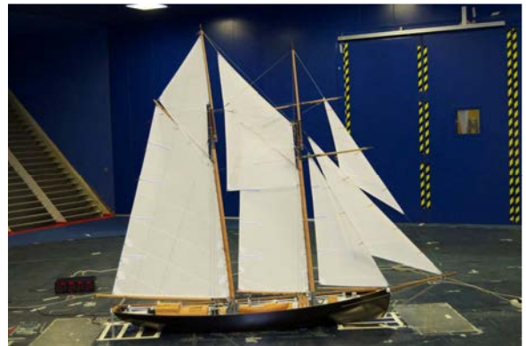
Figure 22 – S3-JT-L-h2 sailplan layout (smaller jib topsail)
