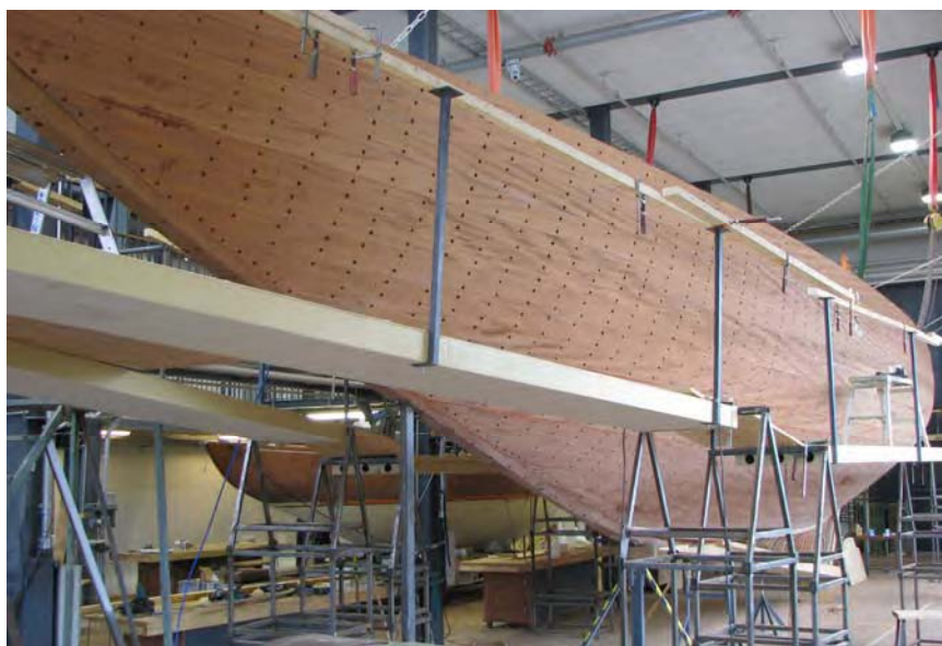
39) Planking installed and sanded, May 2011. Mr. Andersin's Six Metre TOOGOOLOOWOO V is on the far side of the viewing bridge. (Pedrick)
