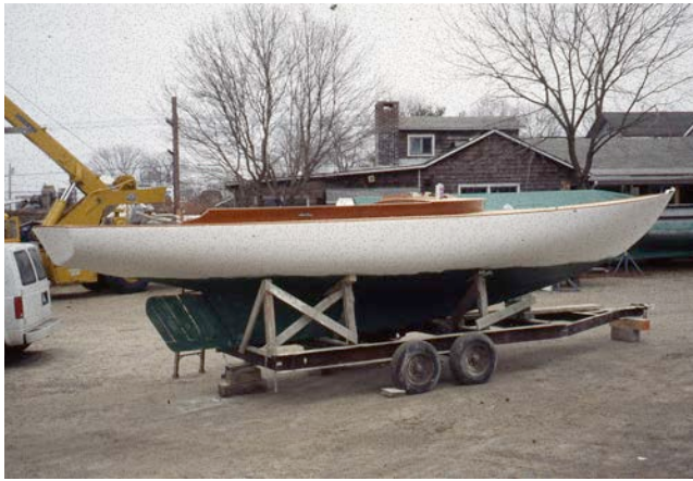
Figure 5- ARIA completed in 1993 without adjustment to restore as designed sheer
