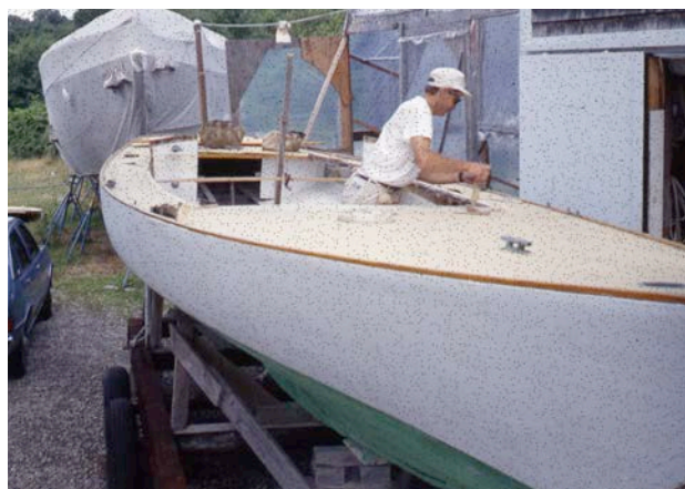
Figure 4- Restoring the deck before fabricating the new cabin
