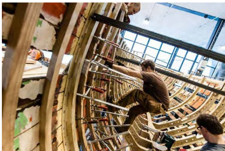
37) Installing steam-bent frames amidships, early 2011. (Skogström)
