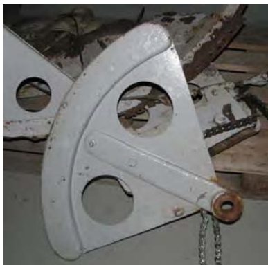
71) BLUE MARLIN's original steering quadrant. (Pedrick)
