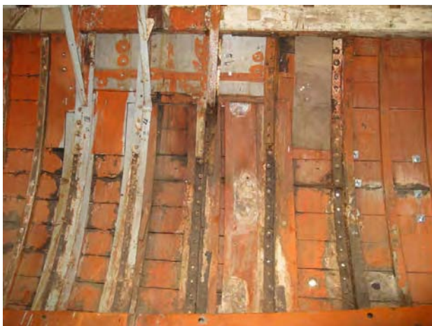
17) Frames in way of the mast and chain plates, port side. Plywood had been inserted between the rusted frames and rotted planks to mitigate leaks. (Pedrick)
