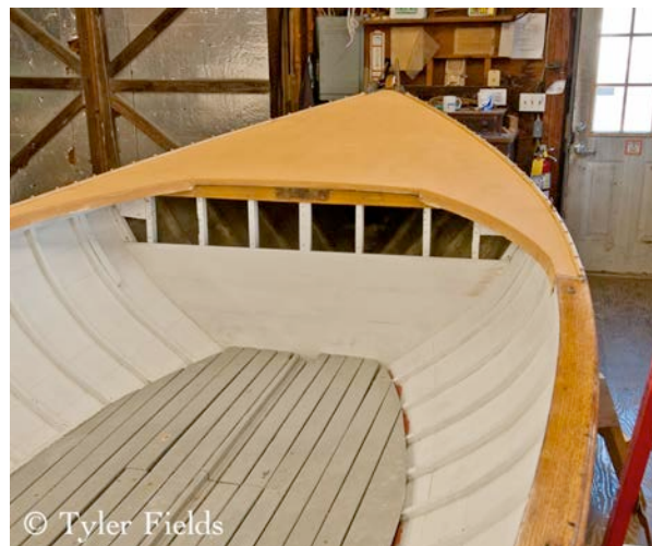
Figure 2- Forward bulkhead returned to the cedar planking and caulked – reopened here for deck work. The original bronze air ventilation holes have yet to be cleaned up and replaced, one at the bottom of the bulkhead and one in the deck just forward of the mast and behind the coaming for through airflow and preservation.
