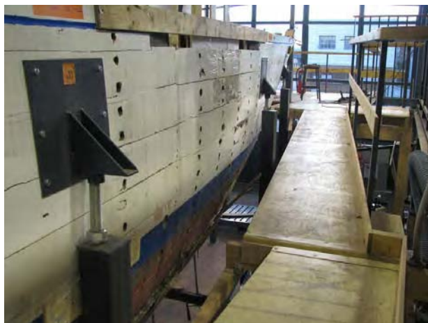
28) Jackscrews bolted to the topsides planking at bent frames were used to align the hull and carry its weight until final installation of all the new frames and floors. (Pedrick)
