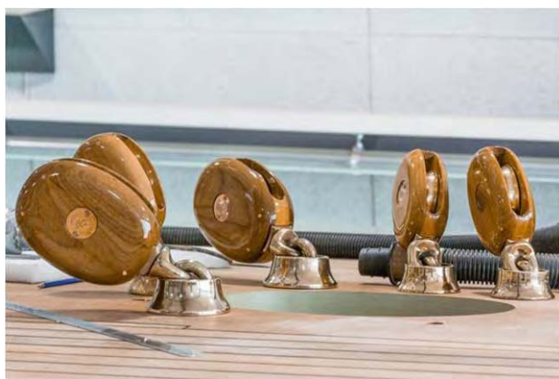
58) Ording blocks with bronze stand-up bases for halyards. (Skogström)
