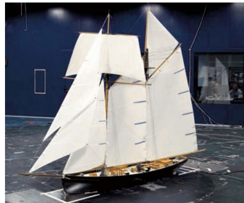
Figure 2 – SALTS schooner wind tunnel scale model
