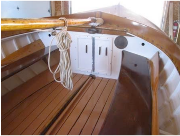
Figure 5 Hand-hole positioned as indicated on the HMCo 1938 revised plans for the H12½ (internet photo).
