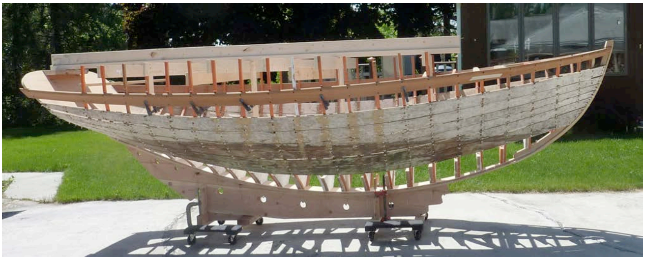
Figure 26 A view of the sheer after the correction. The beam hovering over the boat was my way of keeping the centerline of the boat down the actual center. The beam is attached to the cross members at the remaining molds. It stops at frame eight because the deck beams are already installed up forward.
