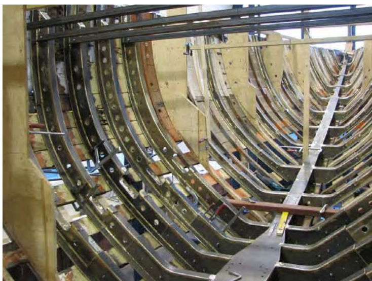
31) Robust web frames at the mast step and chain plates. Original frames had shallow depth, passing between the hull and bilge stringer. New frames are to the full depth of the stringer, with bridge plates bolted across the stringer after it was installed. (Pedrick)
