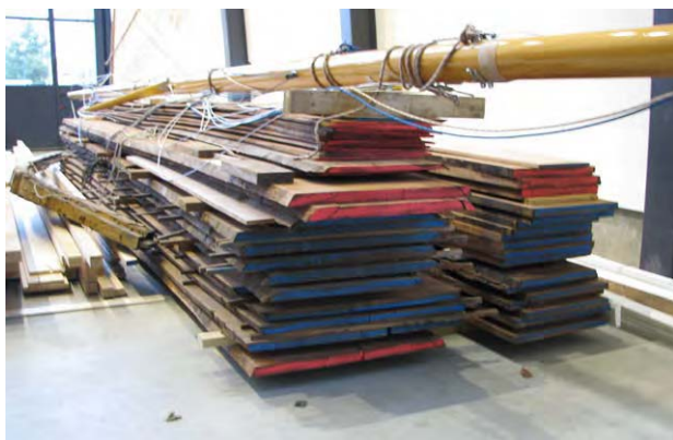
23) Mahogany, drying in the Exhibit Hall of the Wooden Boat Center. Six Metre mast on top. (Pedrick)
