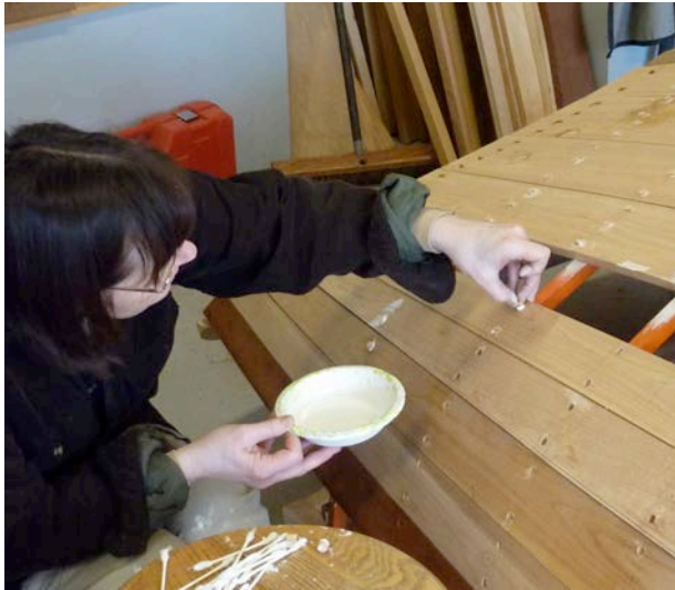
Figure 29 Ann applies paint to the bungs and pushes them into place before lightly tapping them in with a mallet.
