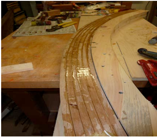
Figure 9 The laminated stem after the clamps were removed; notice the lack of spring- back from the form.
