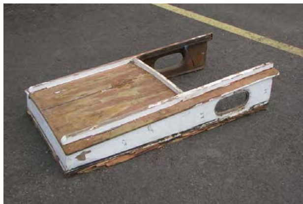
49) Original companionway scuttle from BLUE MARLIN. This was replicated to match the deck's other varnished mahogany. (Pedrick)
