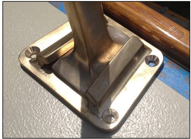
12.) Concordia style stanchion base for ARION.
