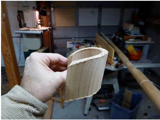
Figure 20 I cut out three nice single piece hounds. I ended up cutting them in half in order to fit them properly around the mast.
