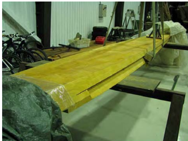
42) The timber keel being shaped in late 2011. To preserve moisture in the wood, the time from wrapped storage to fitting, sealing and installing the keel under the hull was kept to a minimum. (Pedrick)
