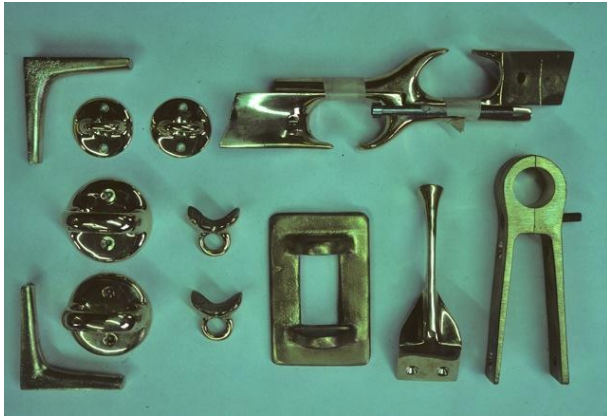
Cast hardware in various stages of completion.
