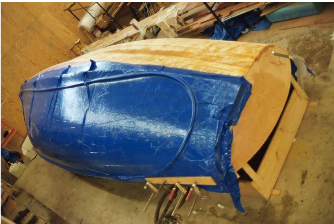
Fig. – 13 Hull Fabrication - Vacuum Bag Applied
