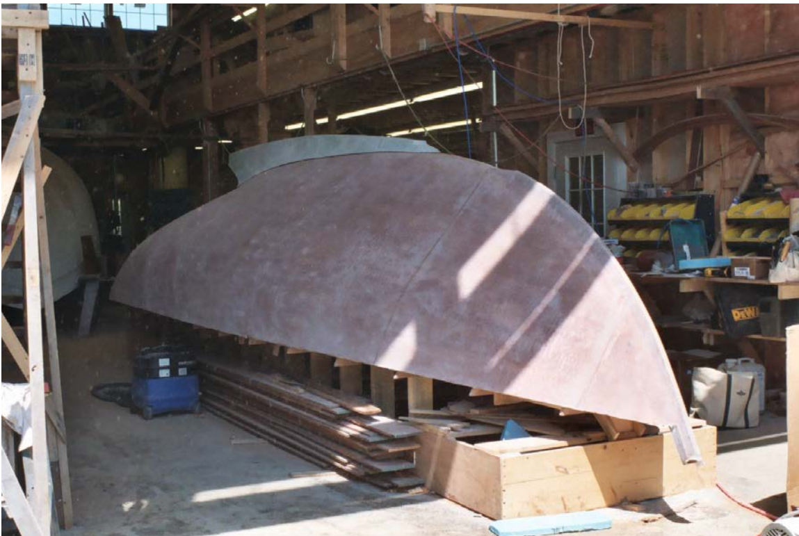
Fig. – 9 Fitting the Ballast Plug
