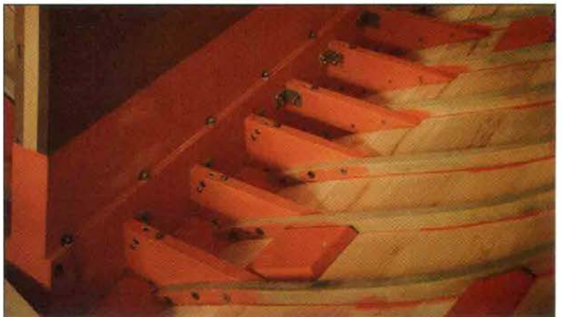
14 The boat turned upright. In the original boat, the butt blocks were fitted tight to the frames, with no chamfer top and bottom. We chose the treatment shown—gaps at the frames and sloped tops—so water would drain.
