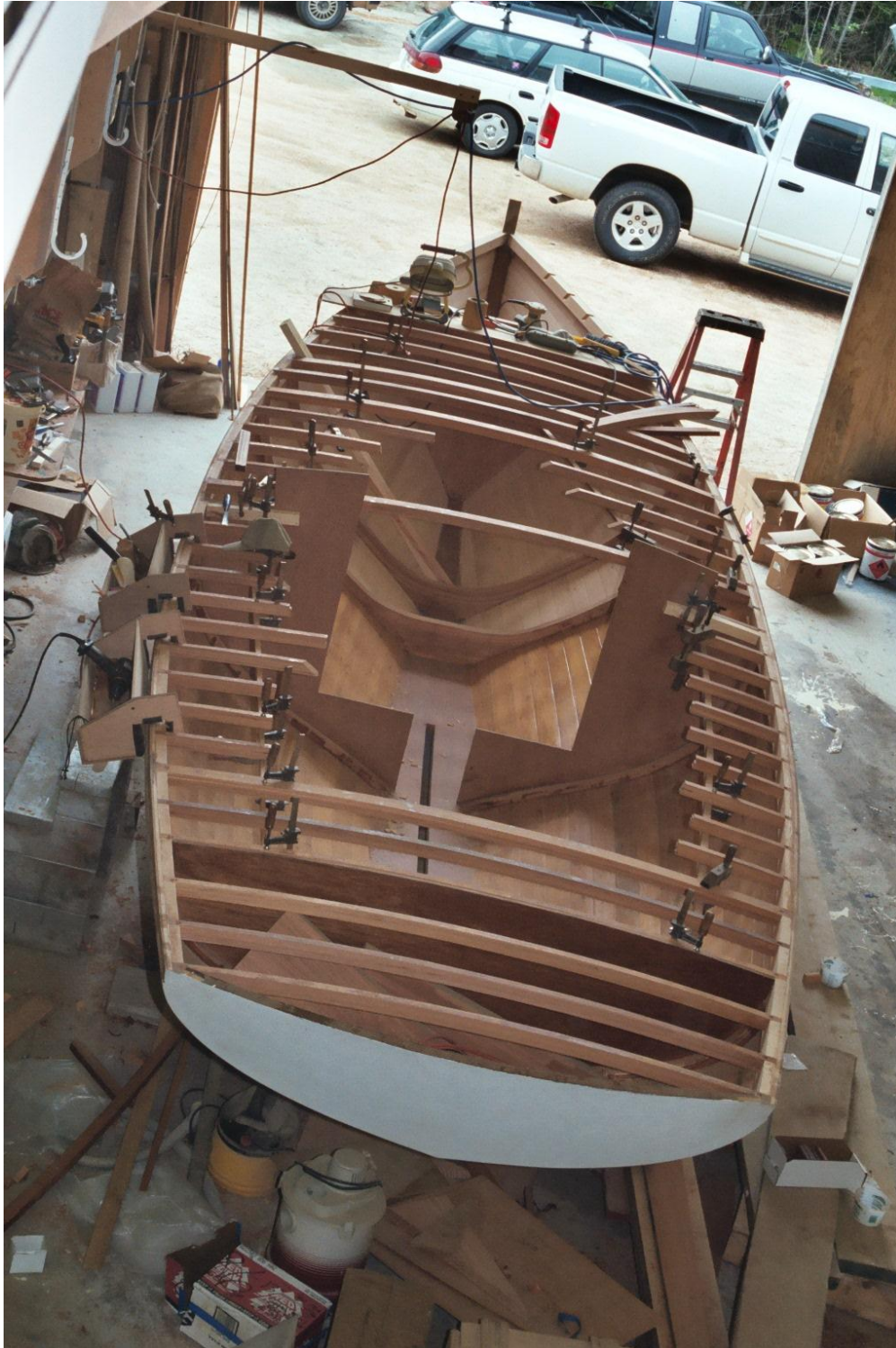
Fig. – 16 Finishing Out – Deck Beams
