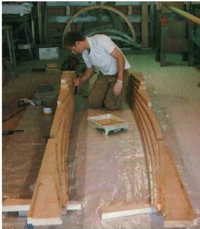
13 The mold for the keel had been built on the loft floor while the planking was underway. This mold consists, essentially, of two "negative half models" formed by waterline lifts and hand-carved to the final shape. The keel was poured and faired in a foundry in Providence, Rhode Island, then refaired in-house.
