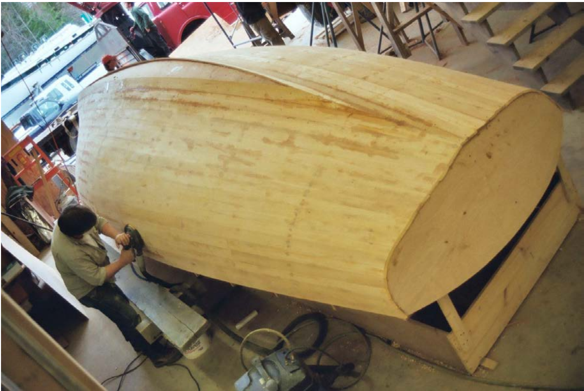
Fig. – 11 Hull Fabrication - Strip Planking
