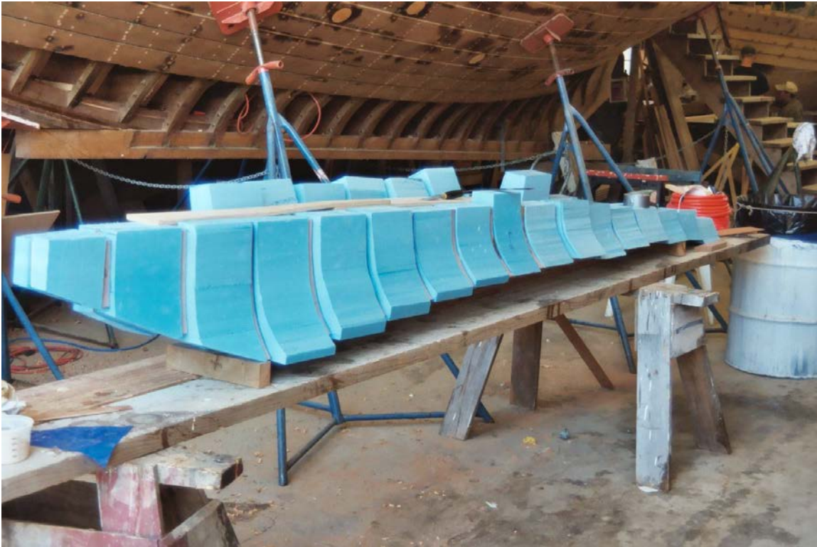
Fig. – 8 Ballast Plug Fabrication
