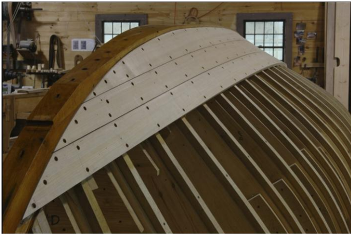
Figure 1 - Herreshoff Method on Molds
