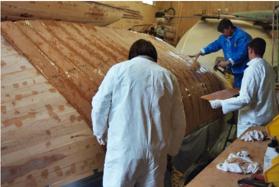
Fig. – 12 Hull Fabrication - Applying Mold Veneers
