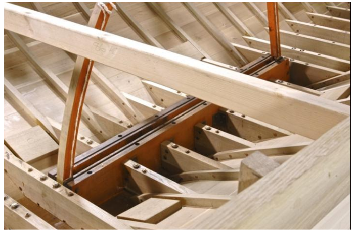
Figure 2 - Interior Molds Removed
