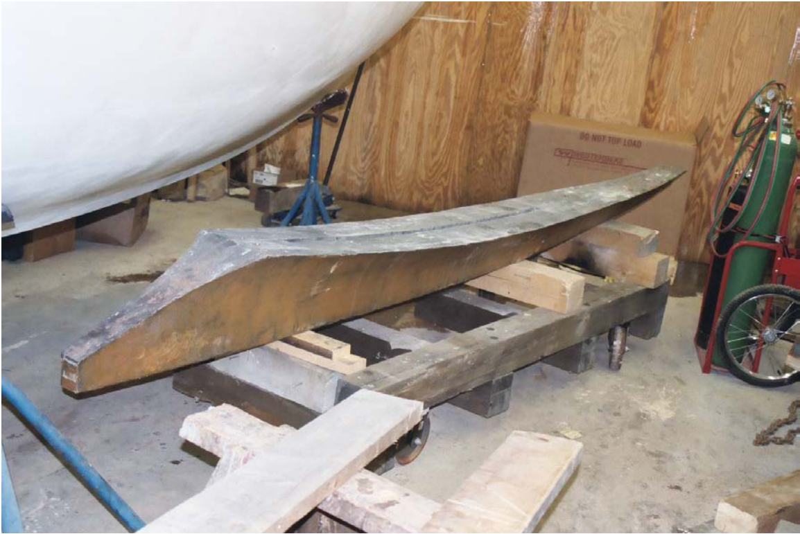
Fig. – 10 Lead Ballast
