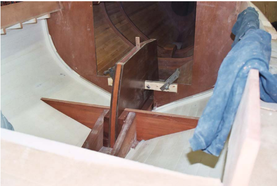
Fig. – 20 Mast Support With Ring Frames
