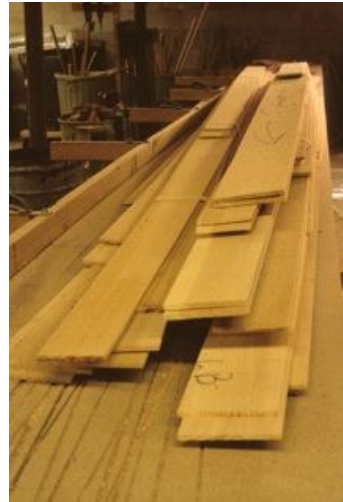
A set of planking, tapered, spiled, cut and marked.
