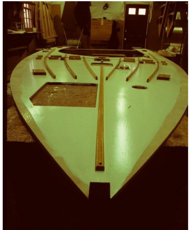
Deck, built upside down on the shop floor with stringers and web blocks installed.
