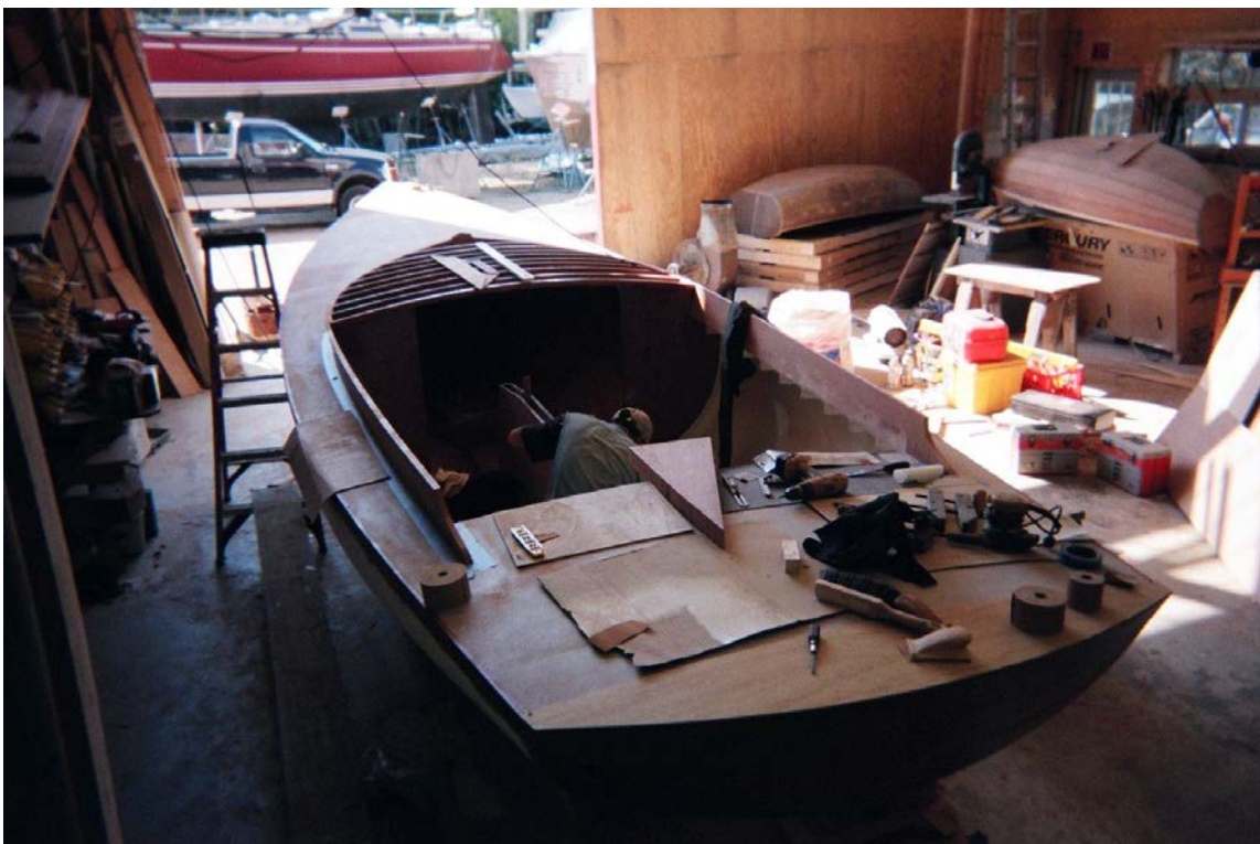
Fig. – 17 Finishing Out –Decks, Cabin, CB Trunk
