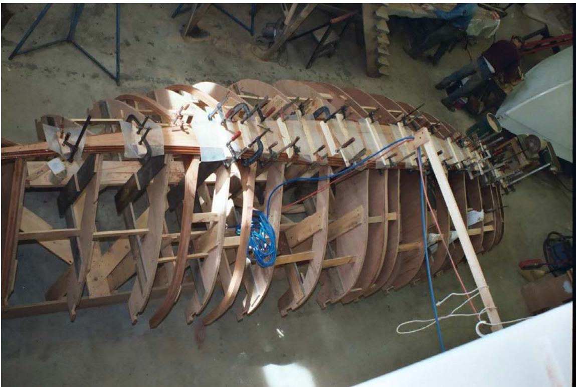
Fig. – 7 Strongback and Mold Setup With Added Boat Components
