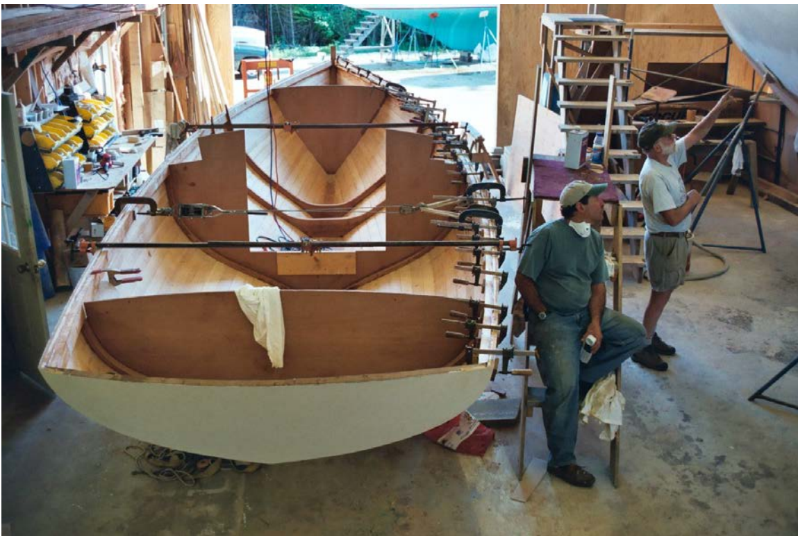
Fig. – 15 Finishing Out – Sheer Clamps
