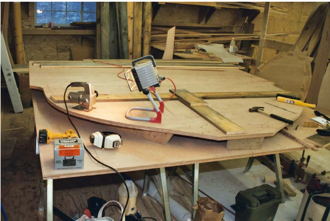
Fig. – 5 Mold Fabrications With Center & Reference Water Lines
