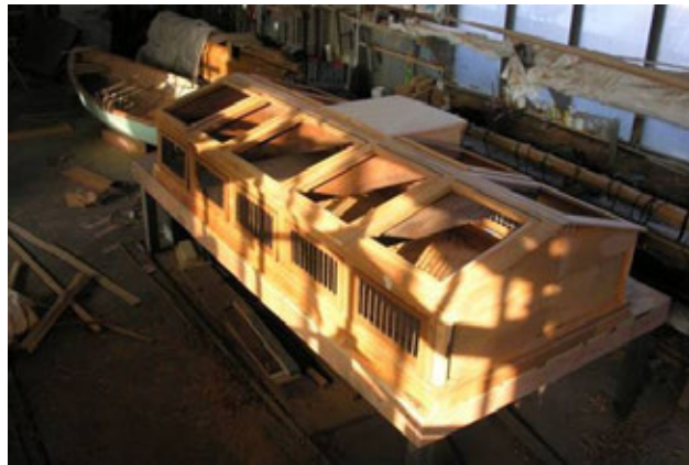
Figure 6- Replication of the engine room skylight showing the grates protecting the side lights.
