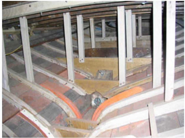
Figure 39 - A forest of additional supports under cockpit.
