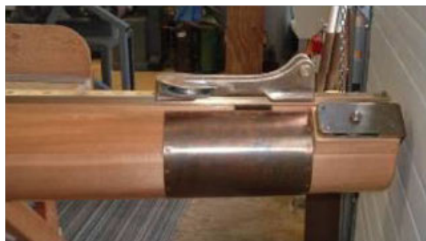
Figure 21 - Original 1912 outhaul car on new boom.
