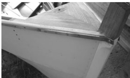
Bronze straps reinforce the stem from the strain of the bowsprit.
