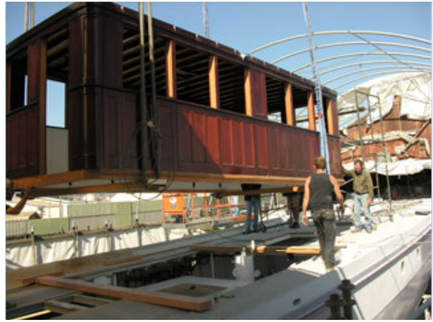
Figure 5 - After cabin being reset on the deck.
