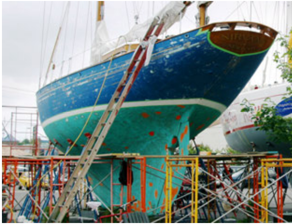
Figure 2 - Filling and fairing the hull.
