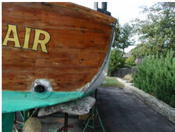
Figure 7 – Starboard transom before removal of exhaust piping
