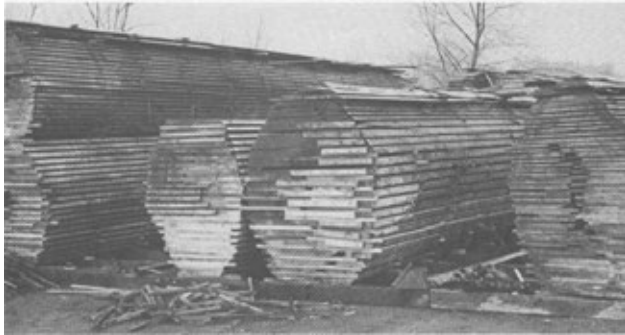
Figure 1 - Whole trees milled and restacked at A&R. ©A Life in Boats – The Concordia Years
