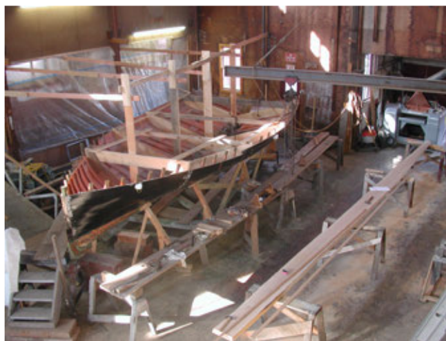
Figure 5 - ANNIE with deck off ready to receive her new plank keel, shown at the right. Photo Kane Borden, Mystic Seaport
