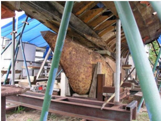
Figure 28 - Ballast keel moved back into place.
