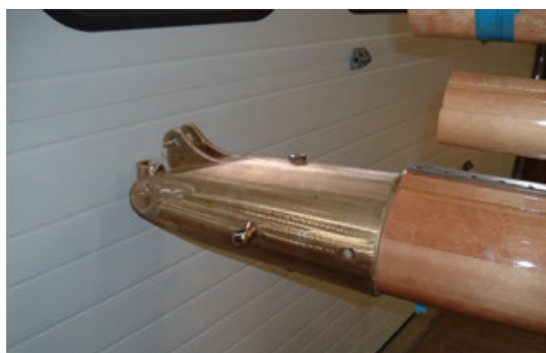
Figure 20 - Original 1912 end bell installed on new boom.
