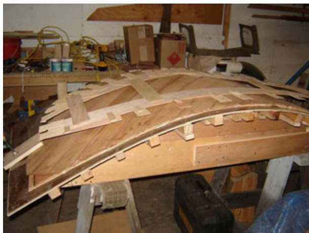
Figure 11 – Three plies of cedar layed over the transom mold.
