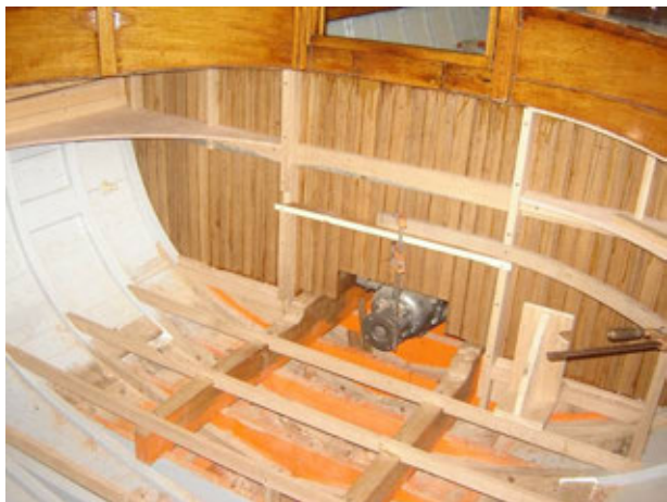
Figure 4 – New tongue and groove midship bulkhead; looking forward. Note cut in the coaming for the door.
