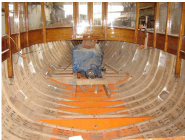
Figure 3- Looking forward from the aft cockpit with the midship bulkhead removed. Illustrates the extremely light hull structure.
