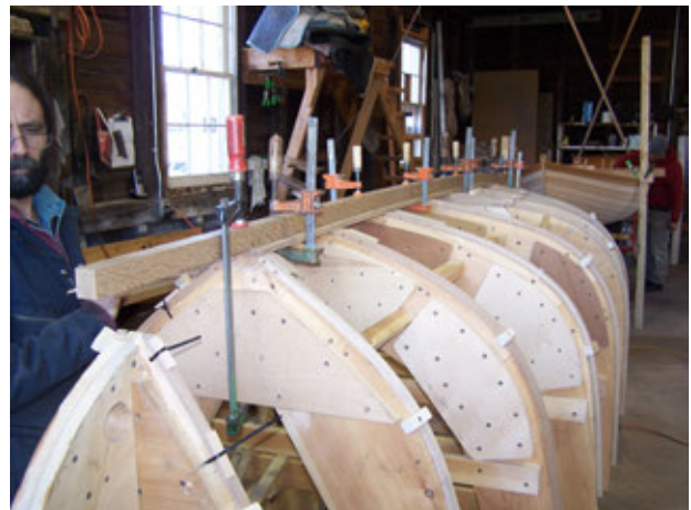
Photo 8- Scott Gifford fitting the keel assembly to the already installed floors and frames.
