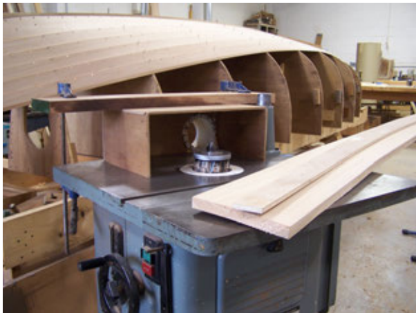
Photo 9 - The set-up we used to produce planks from patterns. The 1/2" plywood plank pattern is shown resting on top of a piece of 7/8" thick Atlantic white cedar planking stock. The shaper cutter behind the plank shows the pattern following bearing above the cutter. A Herreshoff design #404, COQUINA, under construction in the background.
