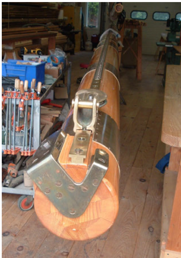
Figure 22 - New outhaul end fitting, sheave and track.
