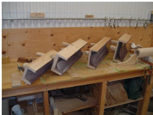
Figure 17 - Sanding boxes for various diameters.
