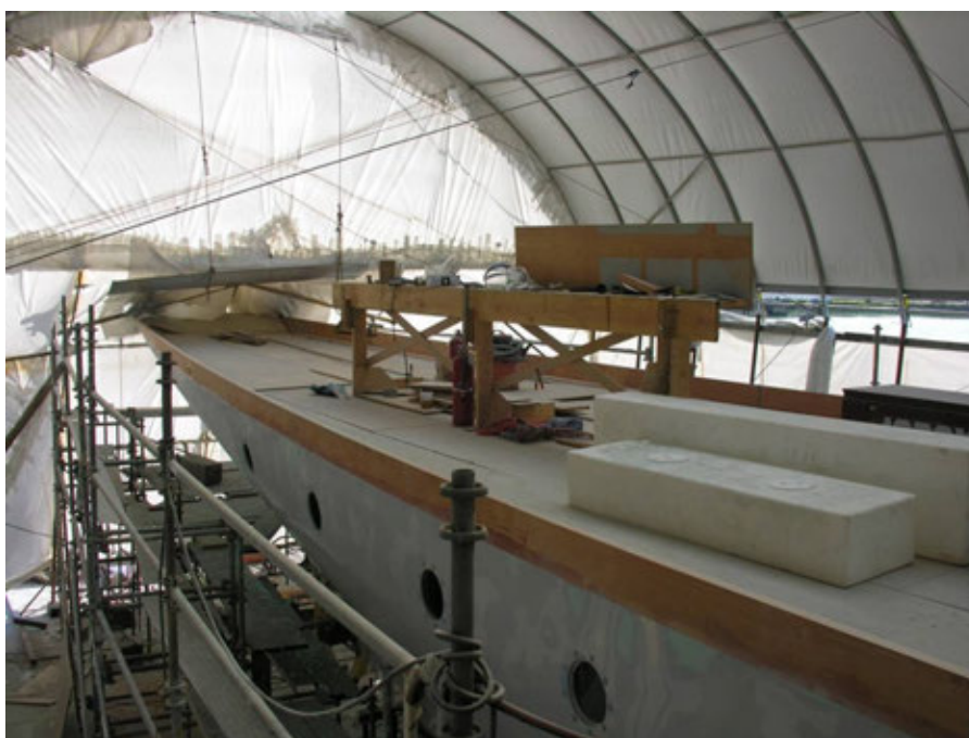
Figure 1 – Hull of CANGARDA showing fairing compound applied and sanded through color layers.
