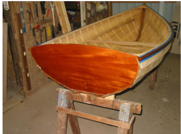
Figure 1 - 2 coats of Clear Sealer applied to transom. This helps seal grain and fill low spots.
