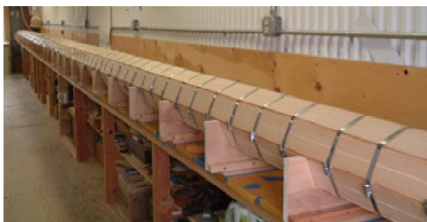
Figure 16 - Spar halves assembled and clamped.
