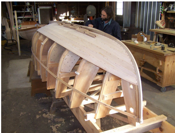
Photo 11- Hull #2 with four strakes of planking on. Scott is adjusting a lap level.
