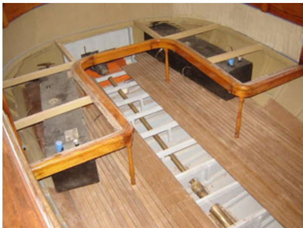
Figure 5 – New seats with fuel tanks below in the aft cockpit- looking forward.
