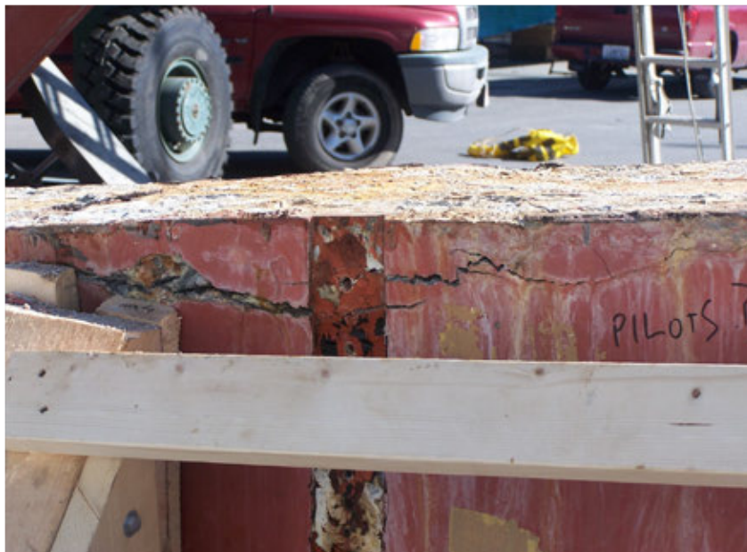
Figure 6 – Mar. '06 – Top of Lead Ballast damaged by water and ice intrusion.
