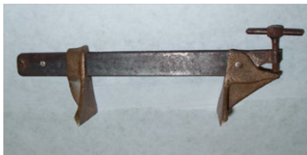
Figure 4 - Herreshoff spar clamp- side view.
