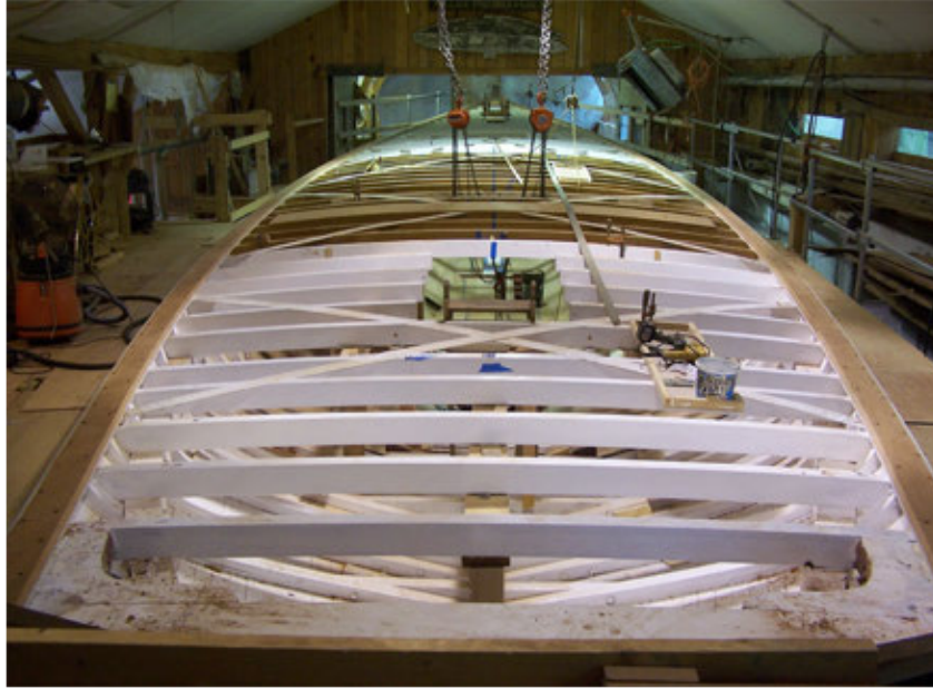
Figure 5A – Oct. '07 – Covering Boards finished.
