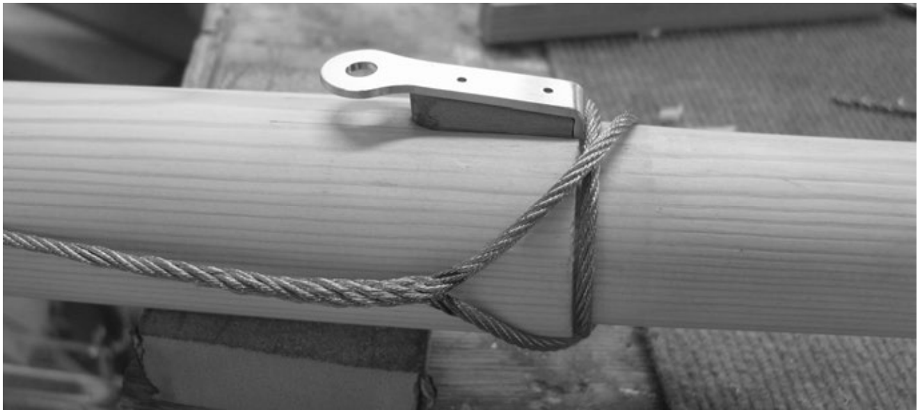
Handspliced bronze mining wire suited RIVIERA's rigging well
