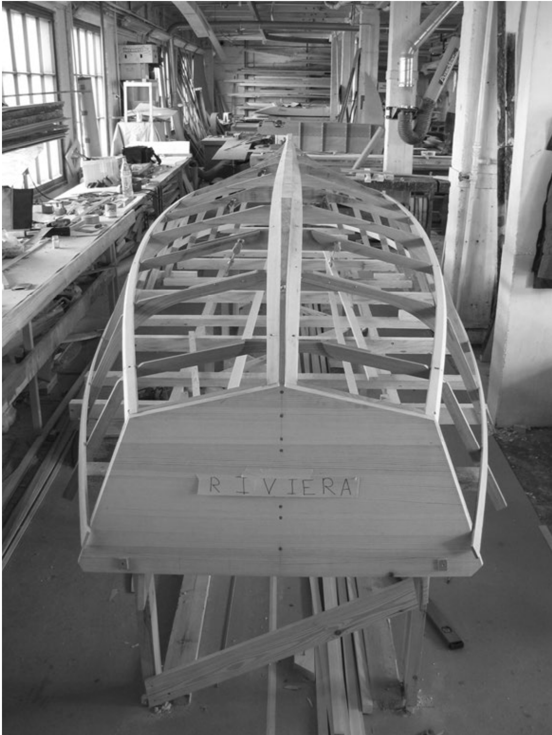
RIVIERA, ready for planking with secondary framing installed.
