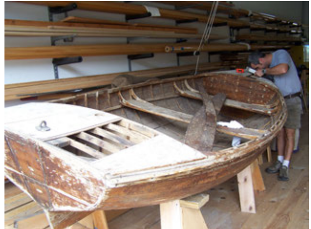
Photo 2- Warren Barker's boat, a 12 ft model of the COLUMBIA lifeboat, with Wade Smith recording construction details
