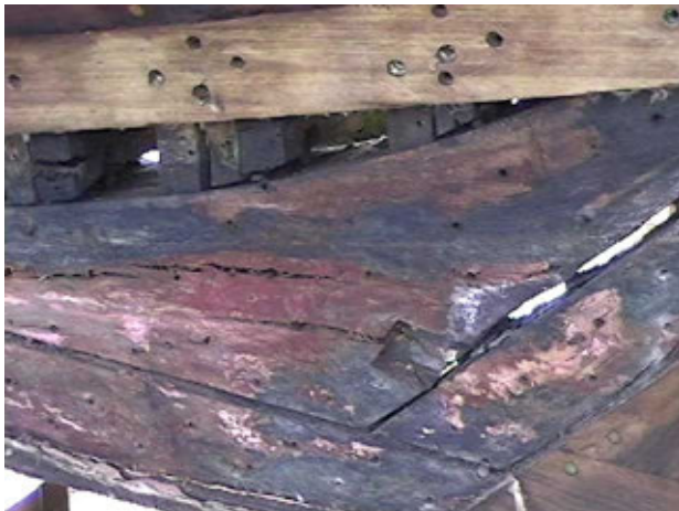
Figure 21 - Twisted and checked stern knee.
