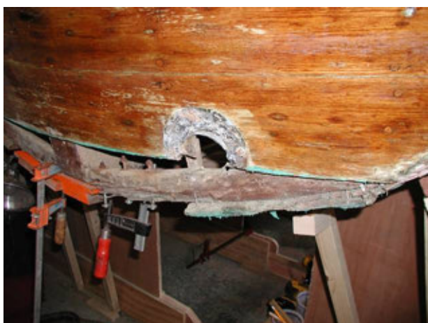
Figure 9 – Damaged cleat shows after removing rotted planking.
