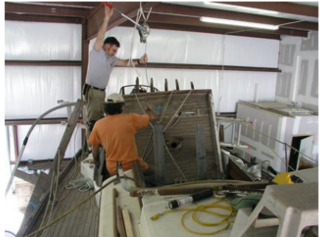
Figure 33 - Extracting the cockpit floor.
