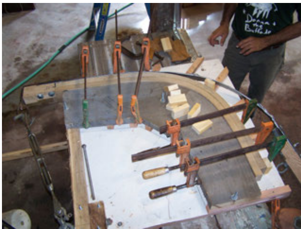
Photo 7- A two-piece, steam-bent, white oak stem clamped to the bending form.
