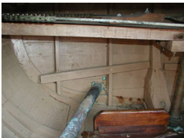
Figure 8 – Interior of starboard transom evidencing rust. Note the double planked transom is fastened from the interior.
