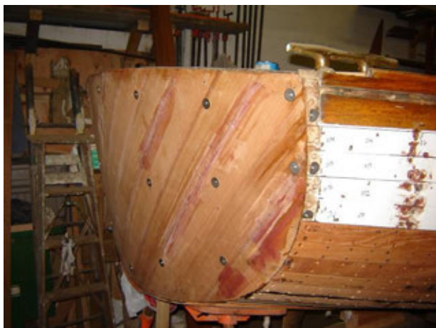
Figure 13 – Cold molded cedar transom in place before teak overlay is applied.
