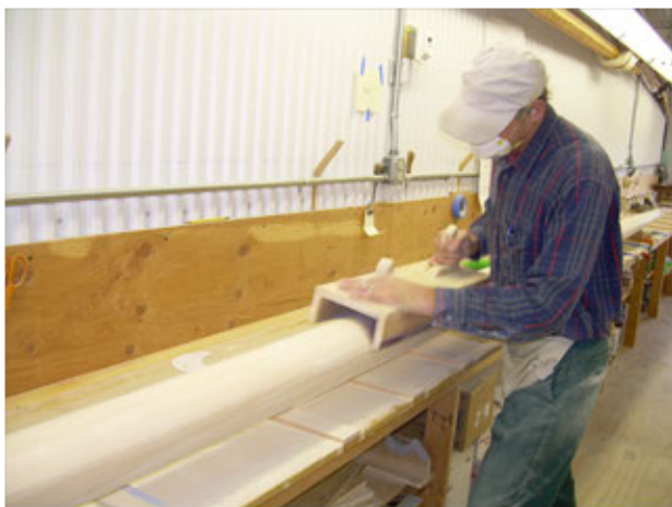
Figure 19 - Shaping spar with sanding box.
