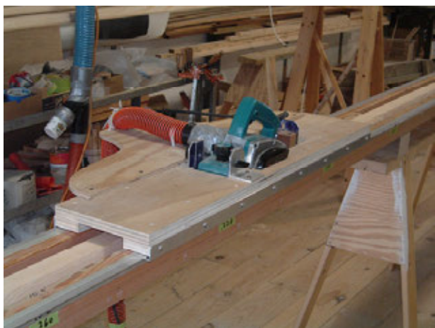
Figure 13 - Power plane and sled on trough.
