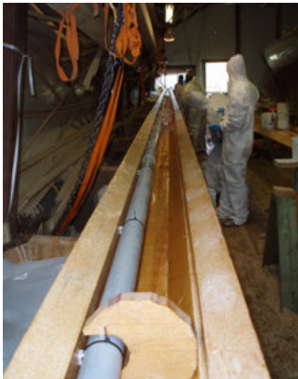
Figure 2- Glue up! Also showing conduit for wiring.
