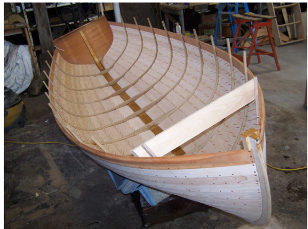
Photo 10- Hull #1 removed from the jig. Plank lap fastenings awaiting riveting...a lot of riveting.
