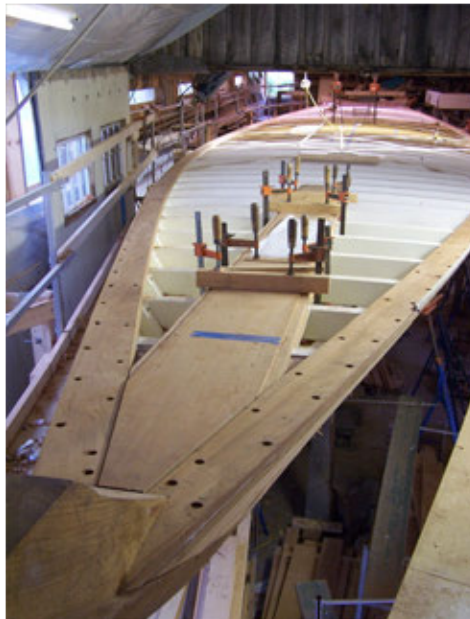
Figure 5B – Oct. '07 – Covering Boards and Fwd. King Plank – Ready for Deacking.
