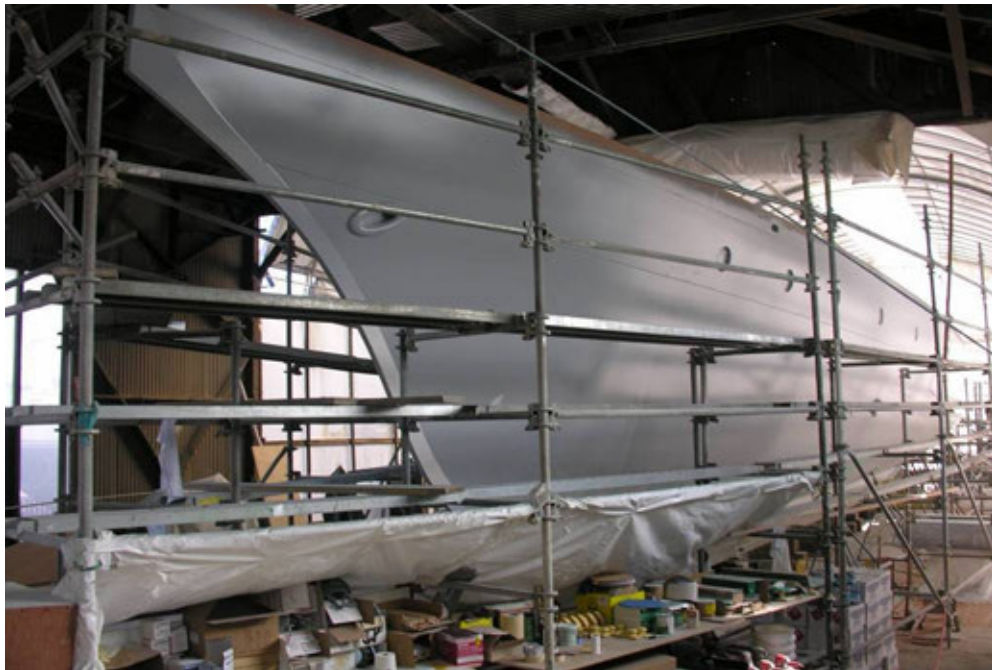
Figure 2 - The hull ready for painting.
