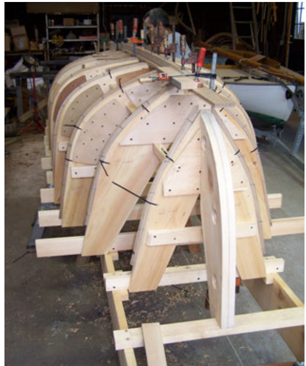
Photo 6- The assembled jig with frames and floors installed.
