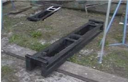
Figure 16 - Beams welded for lifting the boat.
