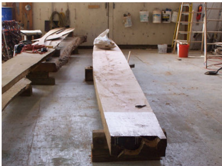
Figure 1 – Aug. '05 – White Oak Keel Timber in MP&G Shop – to Finish 5.4" thick x 25" wide x 28' long clear of Heart and clear of Sapwood.
