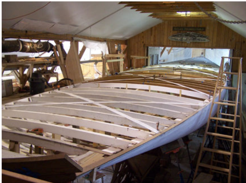
Figure 4 – Apr. '07 – Deck Beams & Straps.
