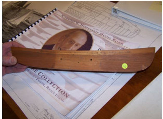
Photo 1b- Notes on reverse side of the half-hull read in part, "Bow changed, sheer raised, re-measured Dec 4, 1909, Boats for 629 and later." Courtesy Herreshoff Marine Museum.
