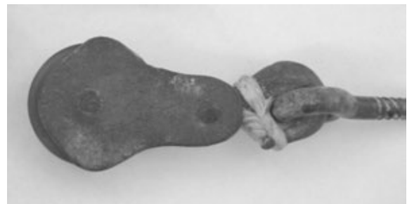
An Original HMCo sheetbronze block
