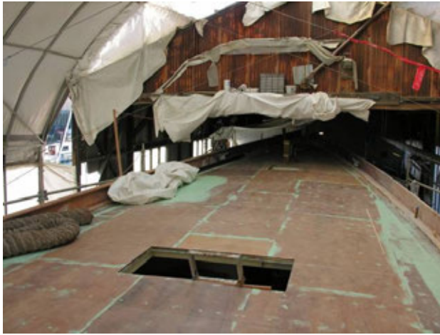
Figure 4 - Deck: two layers of plywood prior to teak.
