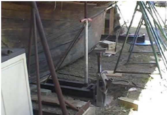
Figure 17 - Railroad jacks used to lift the boat.
