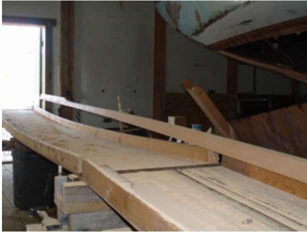
Figure 1- Detail of roller assembly between wooden tray. One finished stave is in the tray
